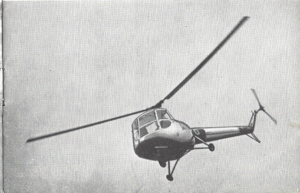
Saunders-Roe Skeeter 2-seat helicopter powered by a Cirrus Bombardier piston engine. Another version of the Skeeter is powered by a de Havilland Gipsy Major piston engine
