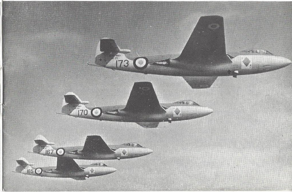
Hawker Sea Hawk single seat naval fighter powered by a Rolls-Royce Nene jet engine
