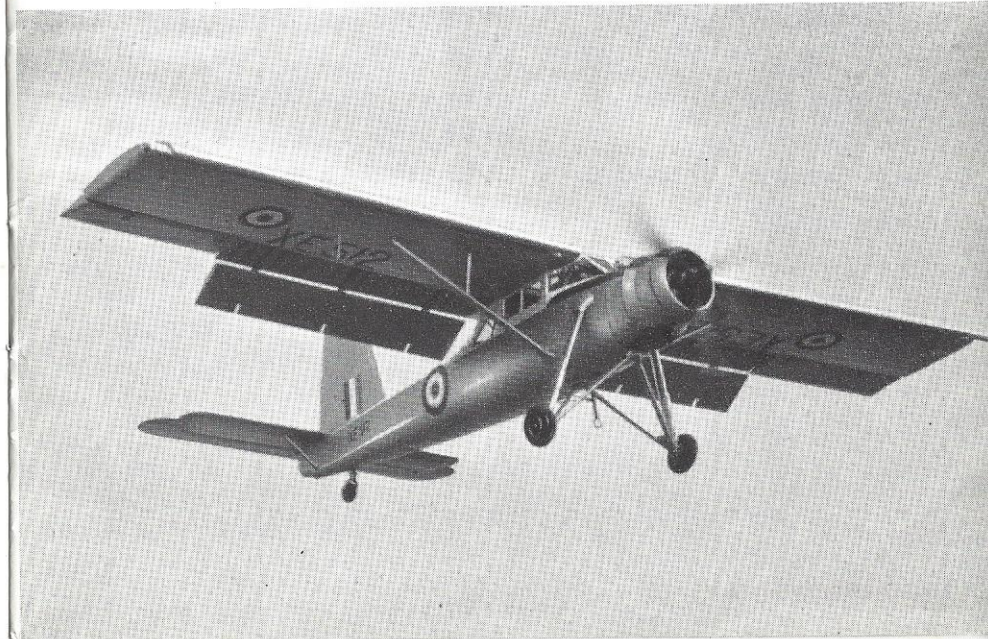
Scottish Aviation Prestwick Pioneer 2 4-seat light transport and ambulance powered by an Alvis Leonides piston engine
