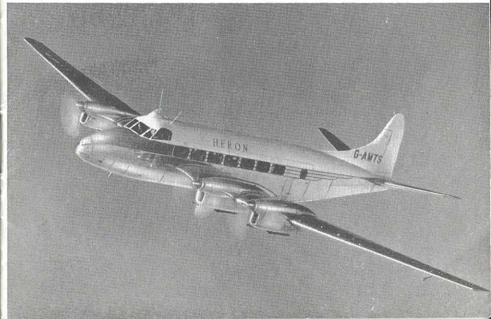
De Havilland Heron Series 2 14-17-seat transport powered by four de Havilland Gipsy Queen piston engines
