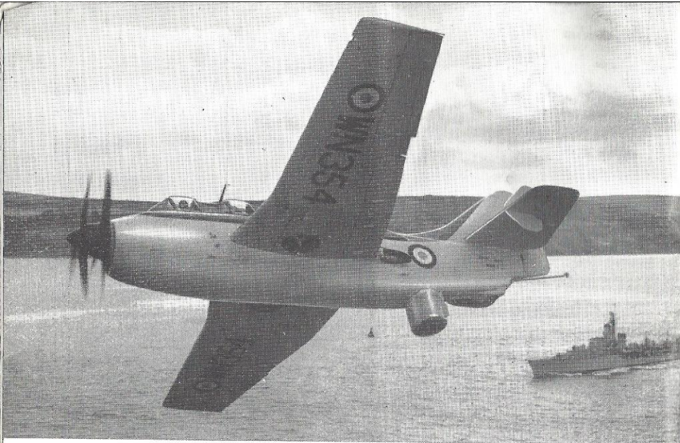
Fairey Gannet carrier-based anti-submarine search and strike aircraft powered by an Armstrong Siddeley Double Mamba turboprop engine
